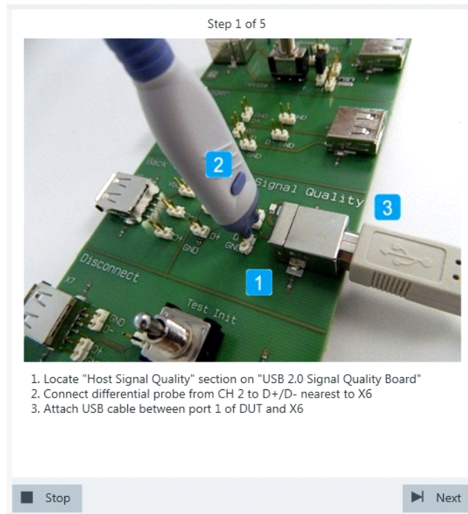
Figure 6-1: R&S RT-ZF1: connection to DUT
