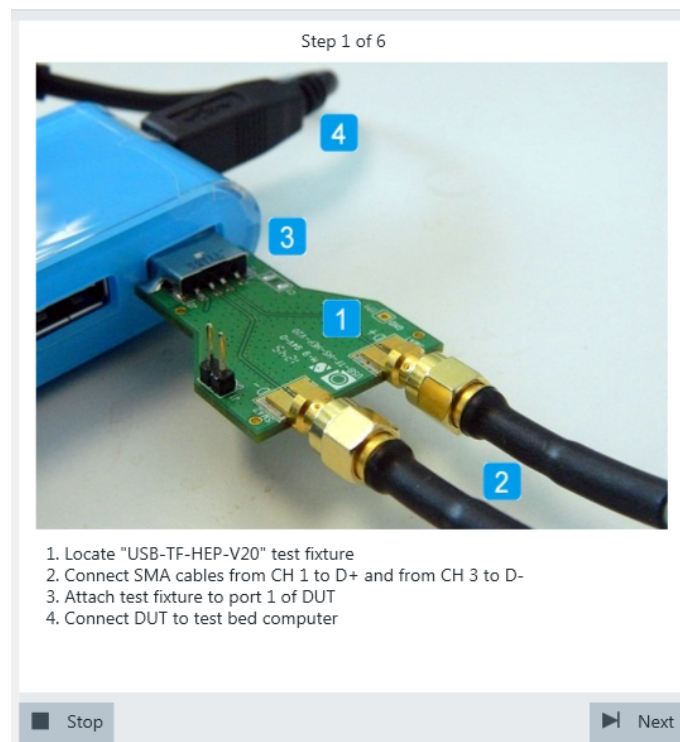
Figure 5-4: USB-IF USB2.0 hi-speed signal quality host test fixture: connection to DUT
