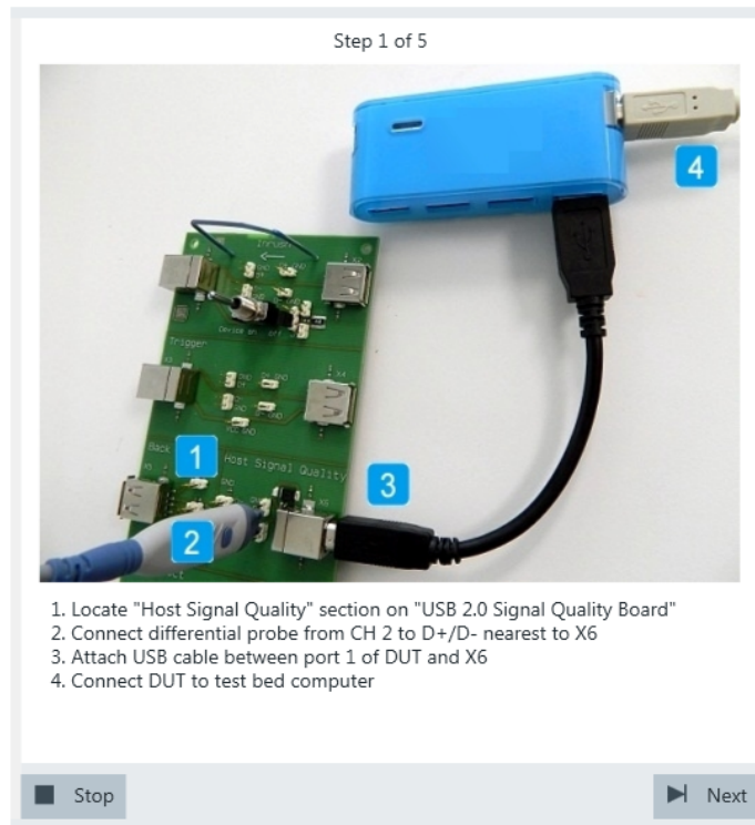
Figure 5-1: R&S RT-ZF1: connection to DUT
