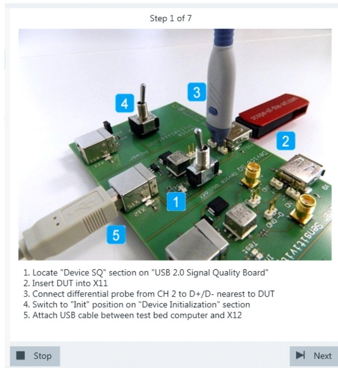
Figure 4-1: R&S RT-ZF1: connection to DUT
