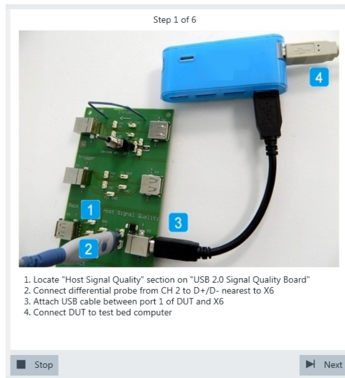
Figure 5-3: R&S RT-ZF1: connection to DUT
