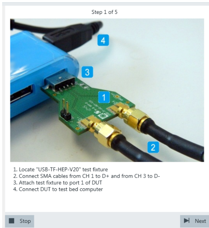
Figure 5-2: USB-IF USB2.0 Hi-Speed Signal Quality host test fixture: connection to DUT
